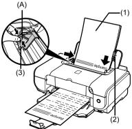
Do not load higher than the Load Limit Mark (A).
